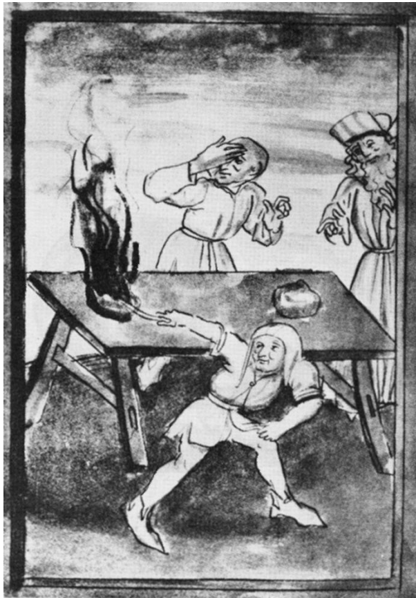
Fig. 1—Testing gunpowder by flashing it on a table. From a Viennese manuscript, 1437.
