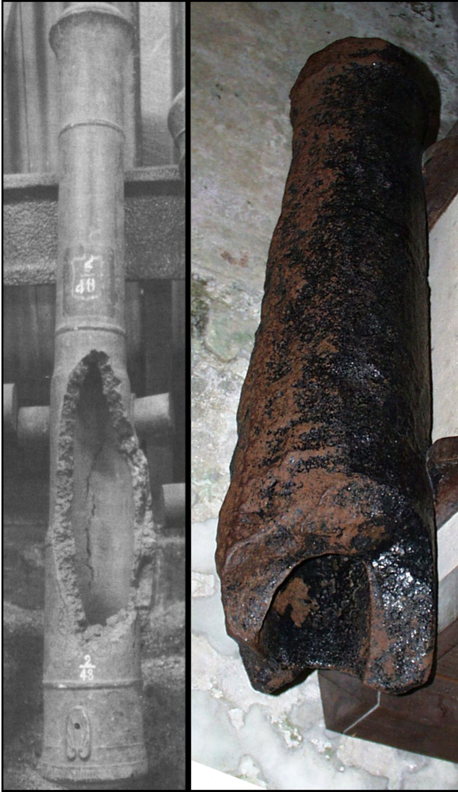
Figure 7. Two guns, one bronze and one iron, that have catastrophically failed (burst). The upper gun is a bronze 6-pdr, cast by Richard Gilpin in 1756 (526 lbs/238.8 kg, 4' 6"/1.372 m long). This English gun burst at St. Lucia in 1783, tearing open longitudinally at the first and second reinforces. Currently housed at the Museum of Artillery Rotunda, Woolwich, from McConnell 1988: Figure 15. The lower gun is all that is left of an iron cannon that exploded, with massive loss of life, while firing on English troops invading St. Augustine on 10 November 1702. Photograph by the author.
