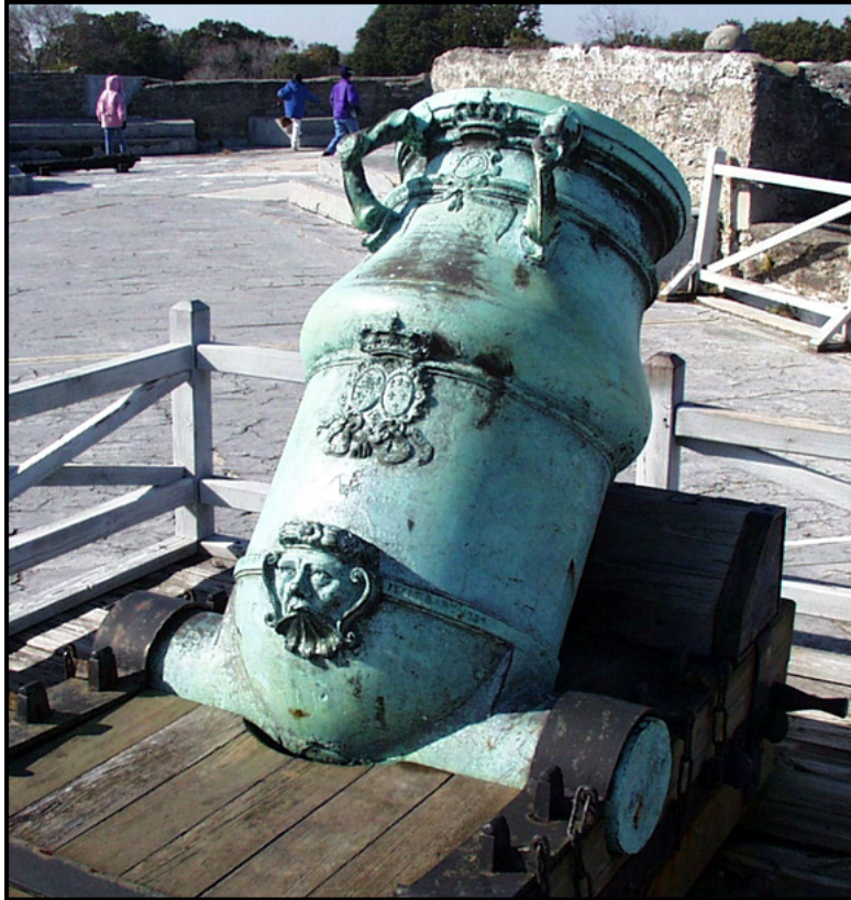
Figure 4. A bronze 15-inch mortar cast in 1724 in Barcelona, captured by U.S. forces in 1898 during the Spanish-American War, and now mounted on a replica bed at the Castillo de San Marcos National Monument in St. Augustine, Florida. Maximum range is listed as 2100 yards or 1.2 miles. Photograph by the author.
