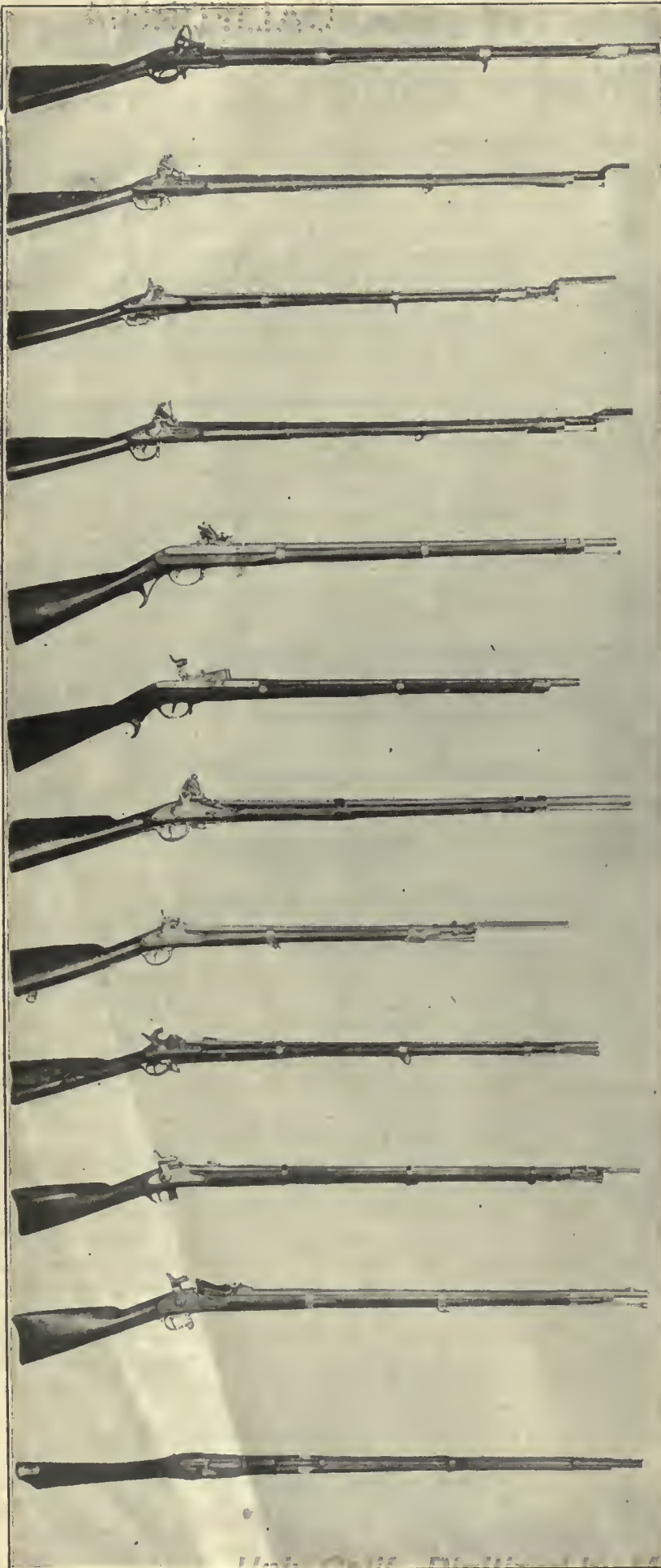
FIG. 3. UNITED STATES MUSKET, 1803 Flintlock; closely resembles French Charleville musket of 1763; made practically as in 1795 and following years at Springfield, Mass.; 71 cal.; diameter of breech, 2 3/4 in.; diameter of muzzle, 7/8 in.; length of barrel, 42 in. (barrel of 1809 musket was 45 in. long); entire length, 56 1/2 in.; weight complete, 10 lb. 7 oz.; without bayonet, 9 lb. 11 oz.; made at Springfield
